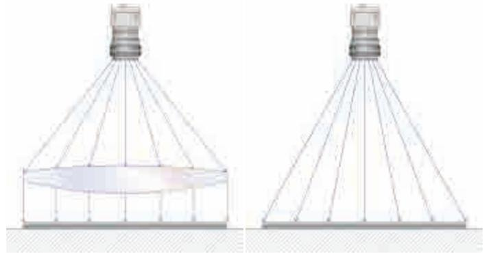
Acquisition of a panel with and without the telecentric lens.
